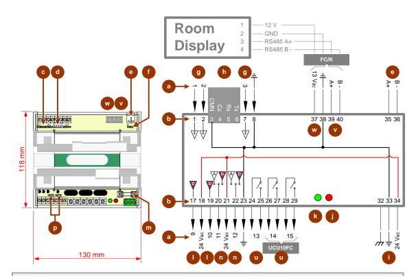
Note: Terminals 18, 21 and 34 are connected internally. When a controller is powered, 24 V AC is available for low current devices at terminals 18 and 21. The total combined current must be less than 1.8 A.
