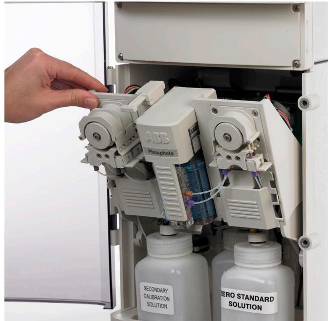
Figure 1 Liquid handling section
