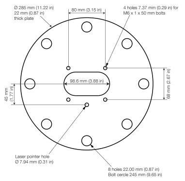
Figure 10 DIN 150 mounting flange (F215)
