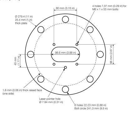
Figure 6 6 inch/DIN 150 mounting plate (P206)
