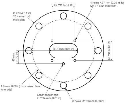
Figure 8 6 inch raised face mounting flange (F206)
