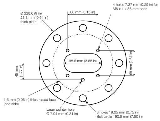
Figure 7 4 inch raised face mounting flange (F204)
