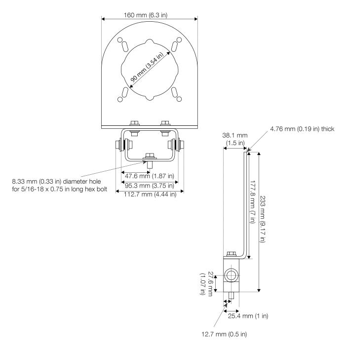
Figure 11 Adjustable pivot bracket (A200)
