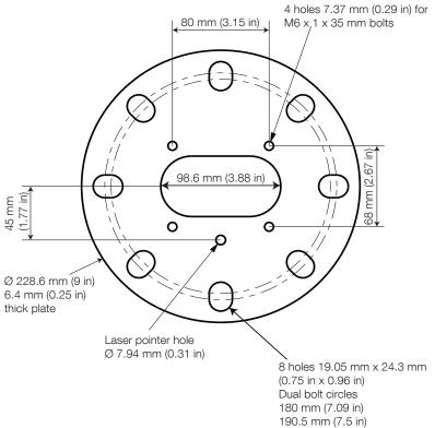
Figure 5 4 inch/DIN 100 mounting plate (P204)
