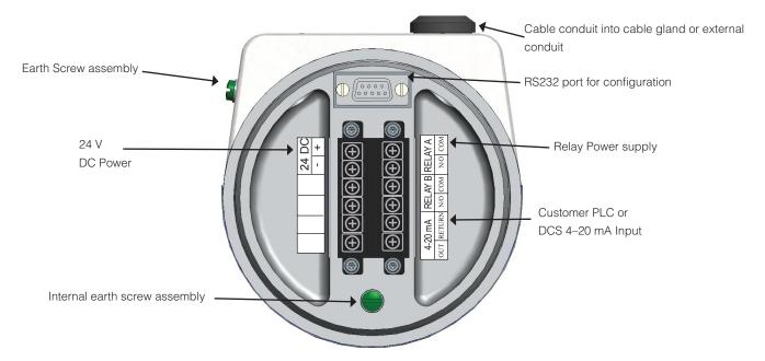
Figure 1 Electrical connections
