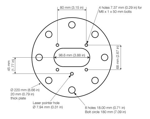
Figure 9 DIN 100 mounting flange (F210)
