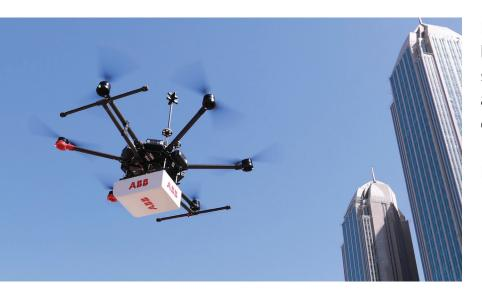
HoverGuard detects natural gas leaks around hard-to-reach sites such as bridges, high-rise buildings, areas with right-of-way restrictions or vegetation coverage, and pipelines.
