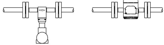
Figure 9: Installation at high measuring medium temperatures
