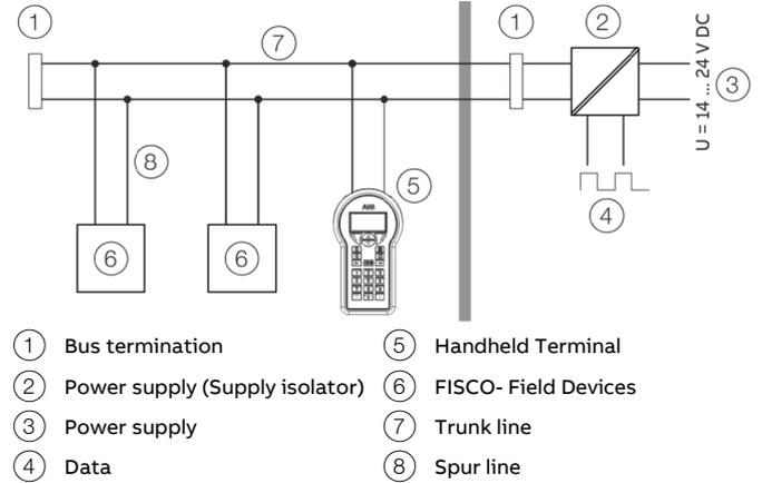
Figure 25: FISCO Control drawing (example)
