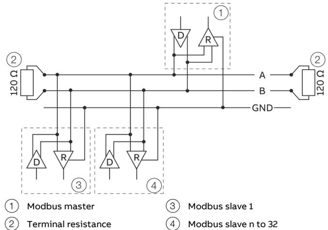
Figure 20: Modbus network (example)
