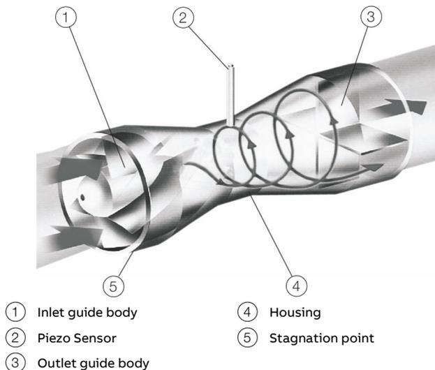
Figure 2: Measuring principle
