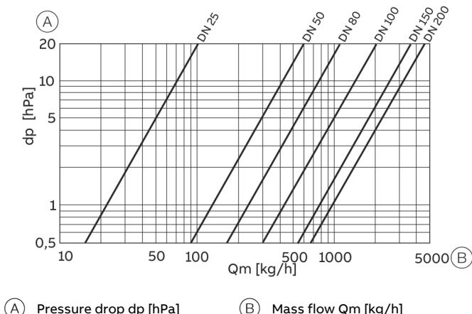
Figure 6: Air filter pressure loss (open)
