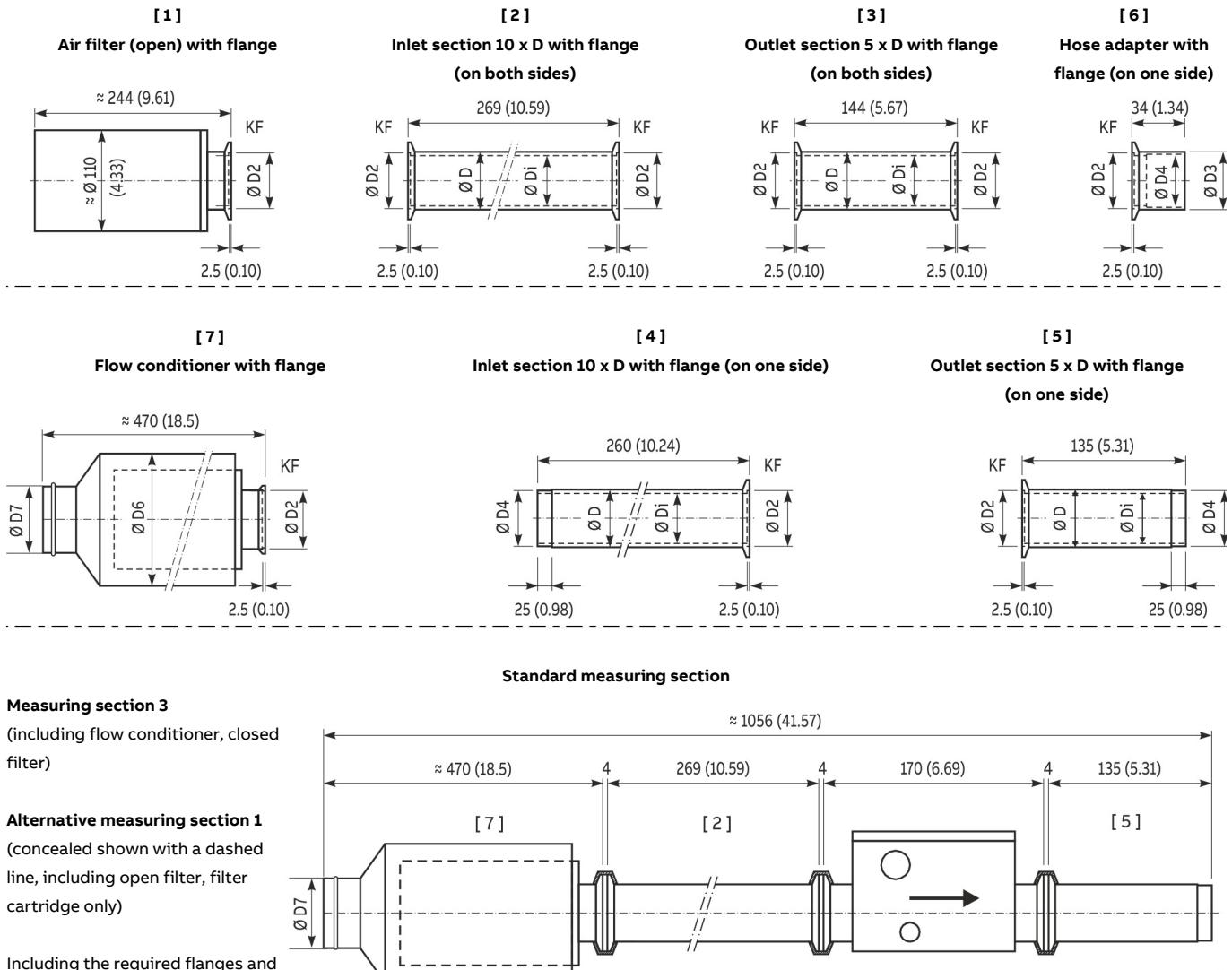
Figure 1: Component dimensions DN 25
