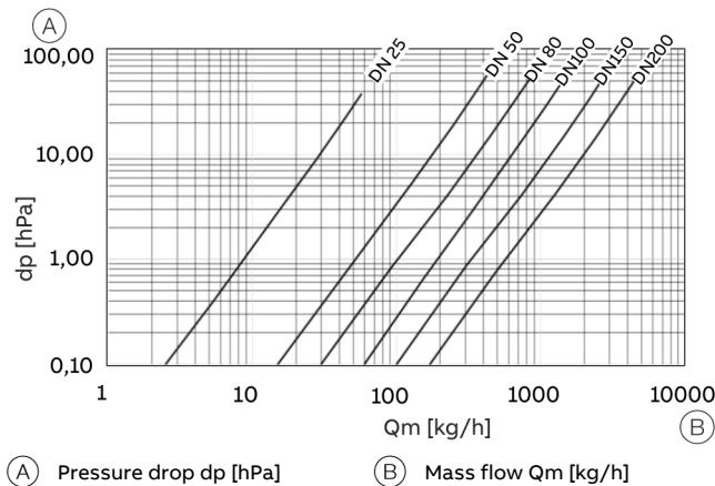
Figure 5: Pressure loss sensor
