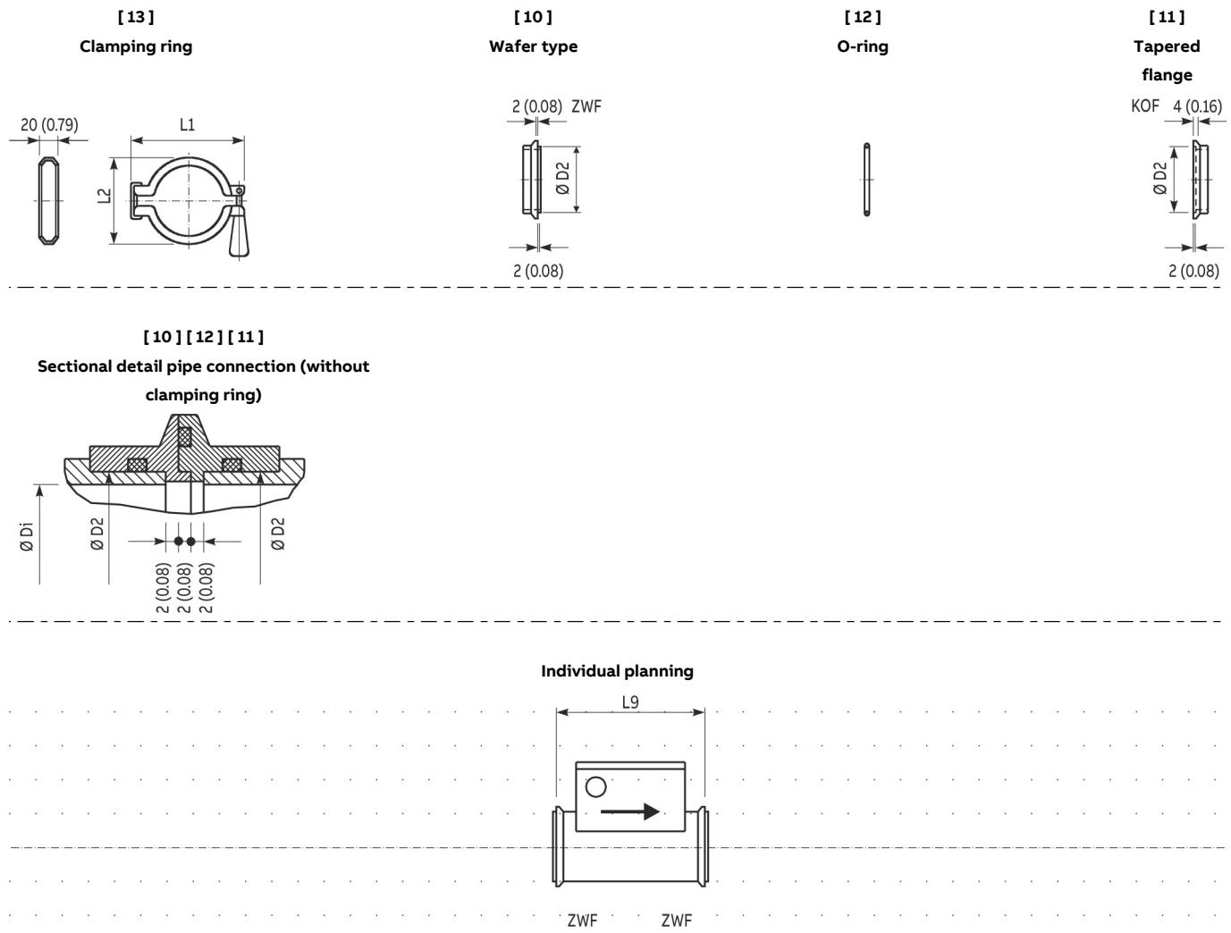
Figure 4: Accessory dimensions DN 50 to DN 100
