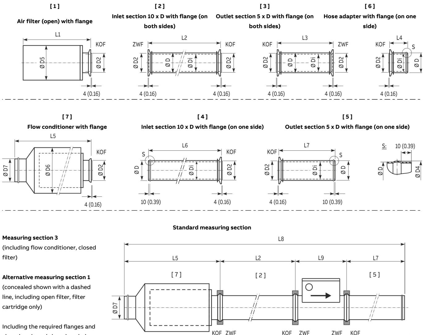
Figure 5: Component dimensions DN 150 to DN 200
