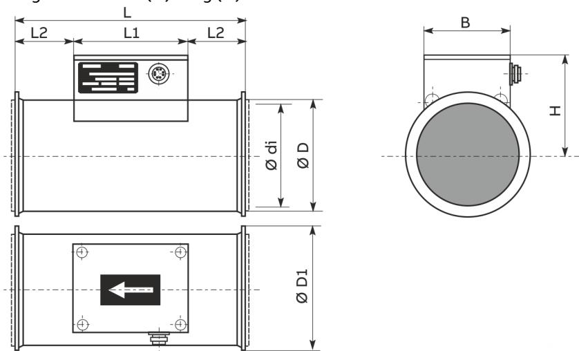
Figure 14: Sensor DN 50 to DN 200
