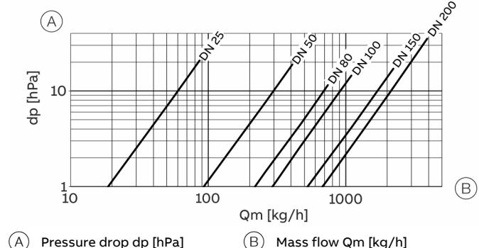
Figure 7: Flow conditioner / air filter pressure loss (closed)
