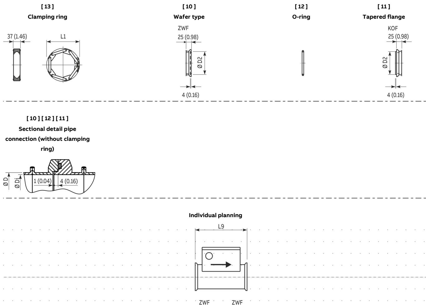
Figure 6: Accessory dimensions DN 150 to DN 200
