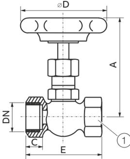
Figure 11: Brass needle valve
