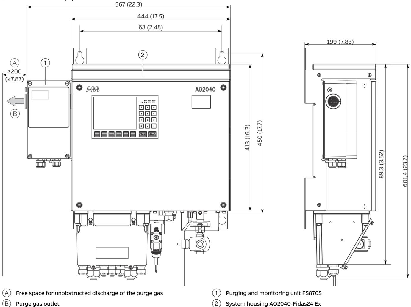
**Figure 27: Dimensions, Model AO2040-Fidas24 Ex****Additional information**
