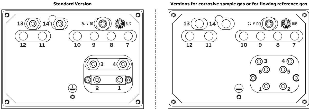
Figure 11: Gas connections Caldos25
