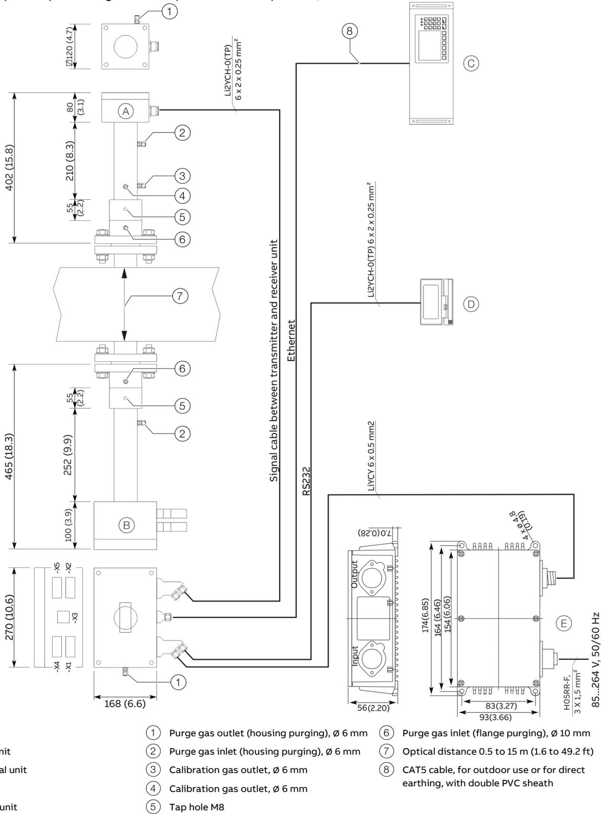
Figure 2: Block diagram of AO2000-LS25
