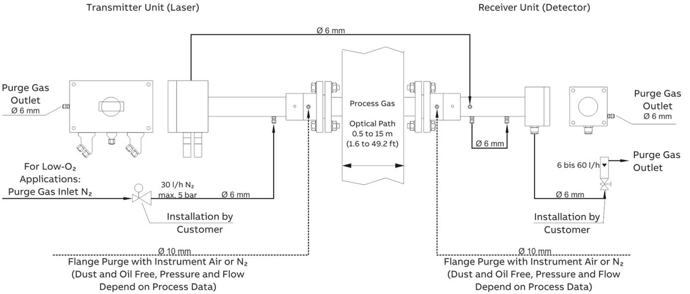
Figure 3: Purging of the transmitter and receiver units
