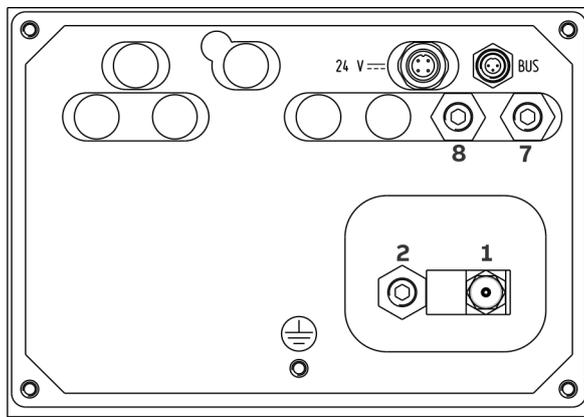
Figure 10: Gas connections Z023
