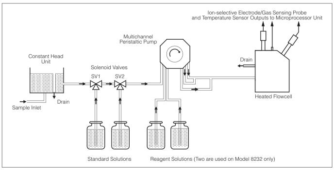
Schematic Flow Diagram
