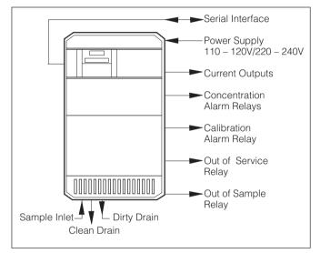
Input and Output Connections
