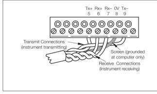
RS422 Connections within Microprocessor Unit
