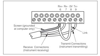
RS423 Connections within Microprocessor Unit
