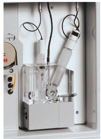
Multi-channel Peristaltic Pump and Sensor Flow Cell
