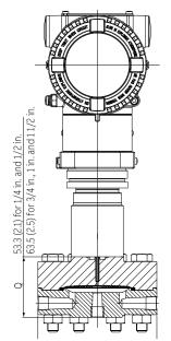
Figure 20 266DRH with barrel housing and direct mount seal S26TT off-line threaded flange
