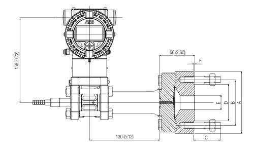
Figure 18 266DRH with barrel housing and direct mount seal S26Mx off-line flanged (For dimensions of S26 seals refer to the S26 datasheet)
