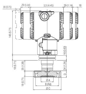
Figure 22 266DRH with barrel housing and direct mount seal S26SS Union Nut (For dimensions of S26 seals refer to the S26 datasheet) Figure 23 266HRH / 266NRH with barrel housing and direct mount seal S26SS Union Nut (For dimensions of S26 seals refer to the S26 datasheet)
