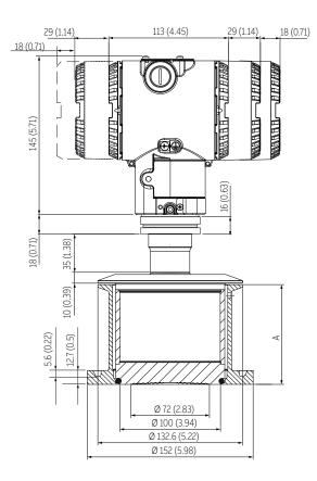
Figure 31 266HRH / 266NRH with barrel housing and direct mount seal S26SS Sanitary extended
