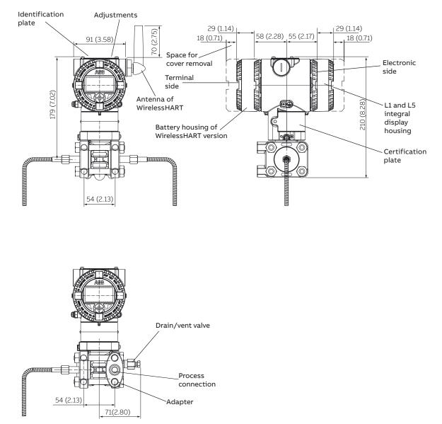
Figure 2 266DRH with barrel housing and remote seal(s)
