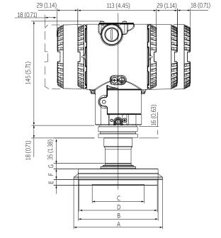
Figure 27 266HRH / 266NRH with barrel housing and direct mount seal S26SS Cherry Burrell (For dimensions of S26 seals refer to the S26 datasheet)
