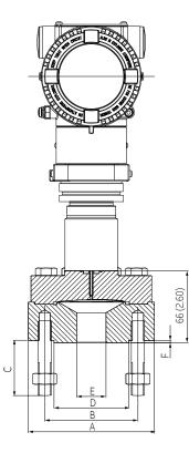
Figure 19 266HRH / 266NRH with barrel housing and direct mount seal S26Mx off-line flanged (For dimensions of S26 seals refer to the S26 datasheet)
