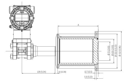
Figure 30 266DRH with barrel housing and direct mount seal S26SS Sanitary extended (For dimensions of S26 seals refer to the S26 datasheet)
