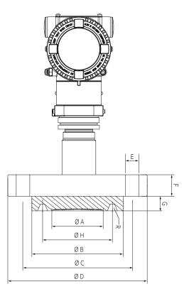
Figure 12 266DRH with barrel housing and direct mount seal S26RR flanged Ring Joint flush diaphragm (For dimensions of S26 seals refer to the S26 datasheet)
