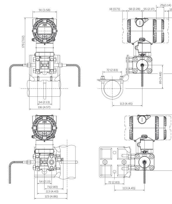
Figure 3 266DRH with barrel housing and remote seal(s) on bracket for vertical or horizontal 60 mm. (2 in.) pipe
