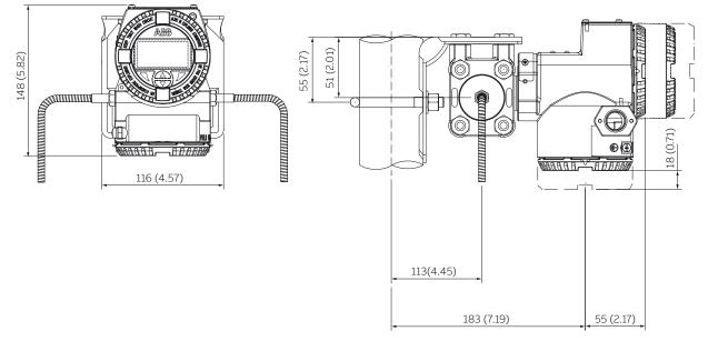
Figure 4 266DRH with DIN housing and remote seal(s) on bracket for vertical or horizontal 60 mm. (2 in.) pipe
