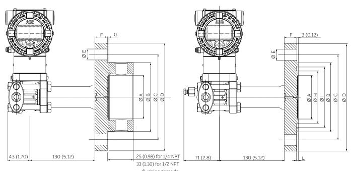
Figure 14 266DRH with barrel housing and direct mount seal S26FA/528FE4FACC<sup>adS</sup> Figure 15 flange Raised Face flush diaphragm ASME and EN 1092/1 smooth and Form B1 (flushing ring as option, only for flush version); Form E (For dimensions of S26 seals refer to the S26 datasheet)
