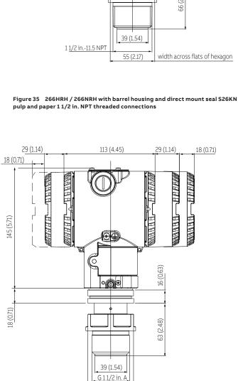
Figure 34 266HRH / 266NRH with barrel housing and direct mount seal S26KN pulp and paper 1 in. Gas threaded connections
