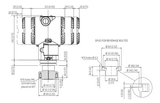
$Figure \ 32 \quad 266 HRH \ / \ 266 NRH \ with \ barrel \ housing \ and \ direct \ mount \ seal \ S26SS \ beverage \ bolted$
