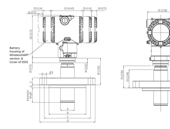
Figure 11 266HRH/266NRH with barrel housing and direct mount seal S26RA/S26RE/S26RJ flanged Raised Face extended diaphragm (For dimensions of S26 seals refer to the S26 datasheet)
