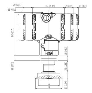
266HRH / 266NRH with barrel housing and direct mount seal S26SS Figure 25 Triclamp (For dimensions of S26 seals refer to the S26 datasheet)
