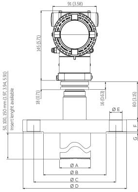
Figure 16 266HRH/266NRH with barrel housing and direct mount seal S26FA/S26FE fixed flange Raised Face ASME and EN 1092/1 smooth and Form B1; S26FE Form E (extension not available). (For dimensions of S26 seals refer to the S26 datasheet)
