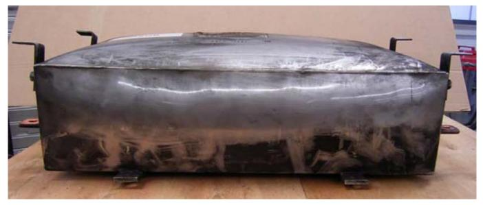
Picture1. Heavy deformation of RFI filter
