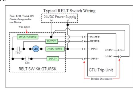
24VDC Power supply – typically this is the auxiliary DC power supply for the trip unit. Whatever DC source supplies the trip unit must also be used for the Input and Output signaling.
