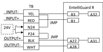
The RELT Switch wires OUTPUT +/- and INPUT +/- will connect to the standard RELT 6 point terminal block that comes with the wire harness.
