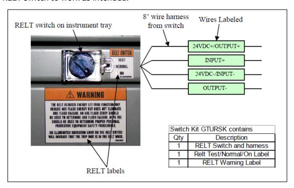
24VDC+/OUTPUT+: This wire is connected to the trip unit positive terminal of the 24VDC auxiliary supply and the trip unit + Output terminal.
