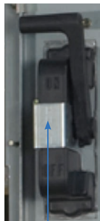
Figure 3. Push in the handle latch
