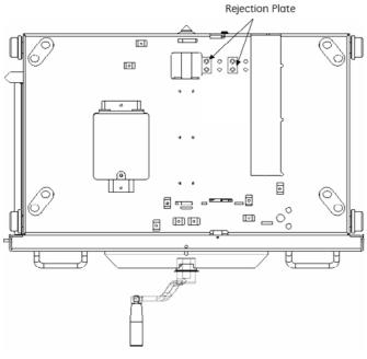
Figure 4-1: Current Rating Interlock, Bottom View
