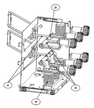
Figure 3-4: Top View, Internal Bus Bar Details
