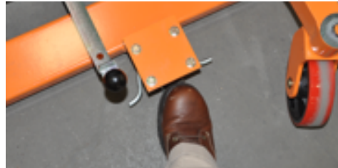
Figure 7. Press the Front Pedal to Lock Lift Truck
