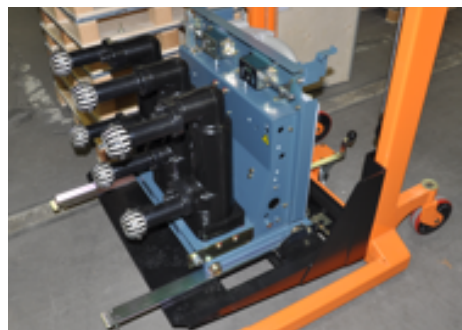
Figure 9. SecoVac VCB Properly Mounted on Lift Truck
