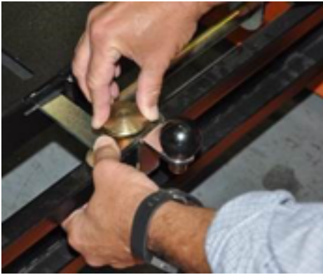
Figure 22. Rotate Interlock Pin Counterclockwise to Unlock the Latch Handle
