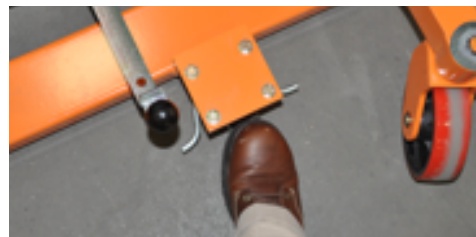
Figure 16. Press the Front Lever to Lock Lift Truck
