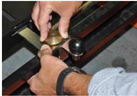
Figure 19. Press Down on the Interlock Pin and Rotate Clockwise to Lock the Latch Handle
