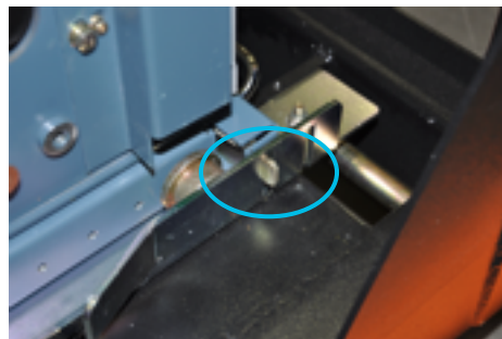
Figure 8. SecoVac VCB Tab Locked in Lift Truck Slot
