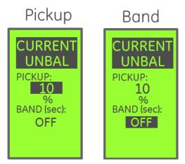
**Current Unbalance** is part of the optional protective relay feature. If protective relaying is not installed on the trip unit, this screen will not appear.
