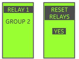
Output Relay configuration **Group 2** links the relay to the overcurrent trip functions (LT, ST, INST, GF, CT GF)
