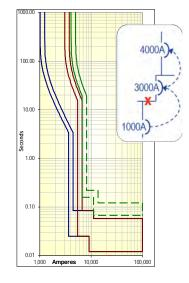
Bus fault – T-ZSI shifts 3000A Pickup to 81%, 4000A Pickup to 123%, and 4000A Delay band per ZSI settings.
