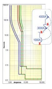
All breakers set for maximum protection. 3000A and 4000A breakers overlap.
