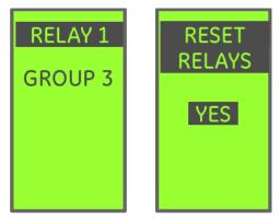
Output Relay configuration **Group 3** links the relay to the Protective Relay trip functions (Voltage Unbalance, Under Voltage, Over Voltage, Current Unbalance, Power Reversal).
