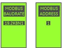
Sets the Modbus communication parameters for the trip unit.
