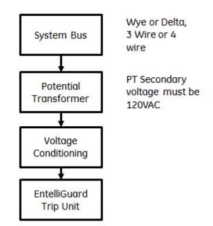
Figure 10-7: Components of an EntelliGuard Voltage Measurement Installation
