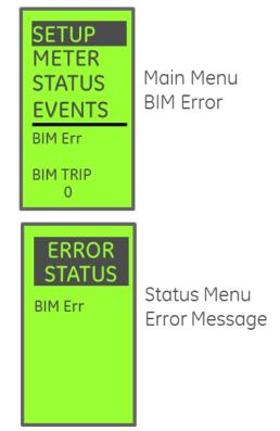
The Breaker Information Module (BIM) is an electronic rejection feature on EntelliGuard G Breakers only. Each time the trip unit powers up it compares its stored information to that in the breaker's BIM. If the data do not match a BIM error condition exists.
