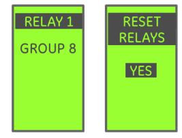
Output Relay configuration **Group 8** (ALARM and TRIP) links the relay to the GF Sum Alarm, GF Sum Trip, GF CT Alarm, and GF CT Trip protection functions.
