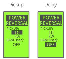
**Power Reversal** is part of the optional protective relay feature. If protective relaying is not installed on the trip unit, this screen will not appear.
