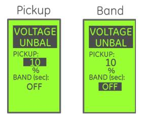
**Voltage Unbalance** is part of the optional protective relay feature. If protective relaying is not installed on the trip unit, this screen will not appear.
