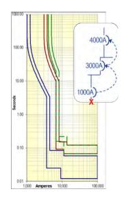
Feeder fault – ZSI shifts 3000A and 4000A delay bands up to allow the feeder time to clear the fault.
