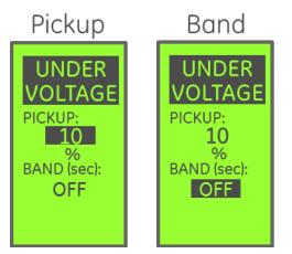
**Undervoltage** is part of the optional protective relay feature. If protective relaying is not installed on the trip unit, this screen will not appear.
