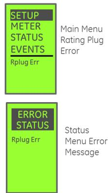
When this error is displayed the trip unit uses its lowest protection settings.
