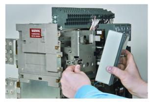
Figure 16-7: Trip Unit Removal Sequence, Step D
