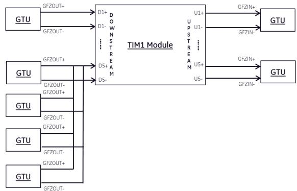
Figure 10-5: Six Trip Units Connected in Parallel to a Single Downstream TIM1 Input Pair
