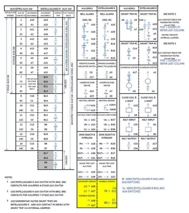
4. Aux contacts B25/B26 and B17/18 are used for Shunt trip 1 and or 2 >125V dc only.
