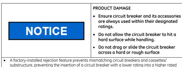
substructure, preventing the insertion of a circuit breaker with a lower rating into a higher ro cassette/substructure, or the insertion of a higher rated circuit breaker into a lower rated cassette/substructure.
