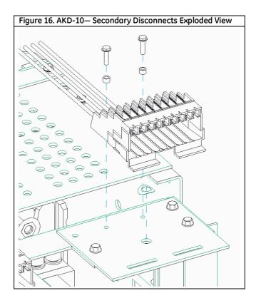
Inputs and outputs to the circuit breaker are wired through secondary disconnects located on the top of the breaker. The plug-style secondary disconnects engage mating disconnects in the breaker cubicle when the breaker is in the TEST or CONNECT position. Up to 72 dedicated points are available so that all breaker accessories can be wired to dedicated disconnect points. Refer to *Table 7* for the secondary disconnect kit catalog numbers.
