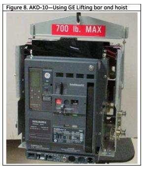
5. Make sure the J hook of lifting bar is secured in the front window on both side sheets of the breaker as shown in fig 8A. This will ensure the breaker is better balanced when lifted.
