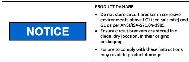
If you decide not to install the Retrofill breaker until a later time, then you can store it away for installing it later.
