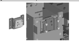
4. Connect the wires via the plug connectors to the respective locations of the secondary isolating contacts A33, A34 and A35 (Fig. 7.18).
