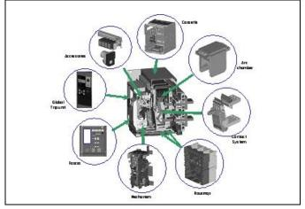
EntelliGuard G circuit breakers consist of rigid front and rear housings made of thermoset composite resins which provide high structural strength and excellent dielectric properties. These housings enclose a contact system consisting of a moving portion and a fixed portion:
