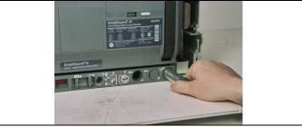
12. Pull out the torque bar from inside the handle and extend (Fig. 3.13).
