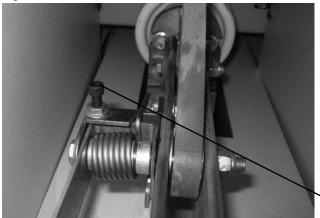
If any corrections in the arcing blade position are necessary (after all previous steps have been completed), loosen the locknut on the arcing blade adjusting screw – see Figure 10 – and turn the screw either in or out to obtain positioning of arcing blade. Re-tighten the locknut.
