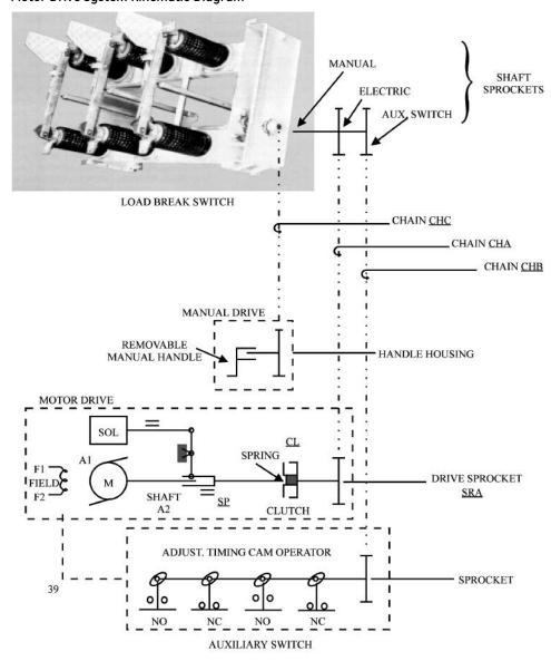
Figure 18 Motor Drive System Kinematic Diagram
