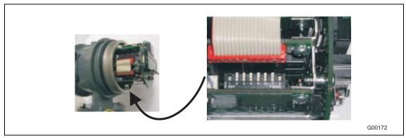
Fig. 54 Position of DIP switches using example of FXE4000 (COPA-XE)
