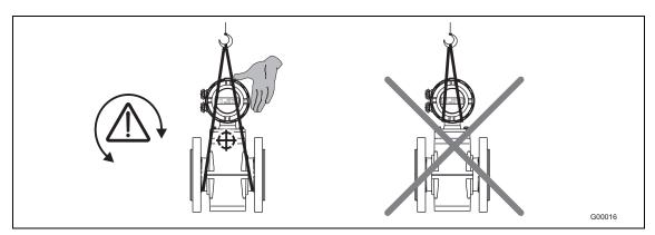
Fig. 8: Transport of flanged units smaller than DN 450
