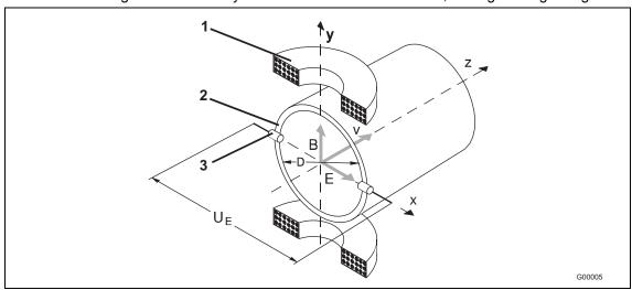
Fig. 5: Electromagnetic flowmeter schematic
