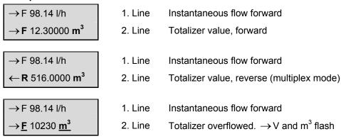
Totalizer overflow always occurs at a value of 9,999,999 units. If the totalizer value for a flow direction is larger than 9,999,999 units, the direction indicators ( $\rightarrow$ F or  $\leftarrow$ R) and the totalizer unit (e.g., m³) flash in the second line of the display. The totalizer software can register up to 250 overflows. The overflow notification can be cleared for both directions by pressing ENTER.
