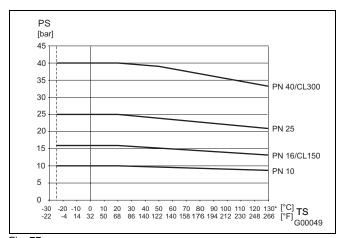
\*) Higher temperatures are allowed for CIP/SIP cleaning for limited time periods, see table "Maximum Allowable Cleaning Temperature".
