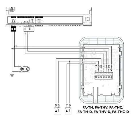
For all controllers, when multiple FusionAir devices are connected to a sensor bus, the power should be connected to an external source:
