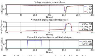
Figure 6. Vector shift algorithm operation during islanding in large power unbalance
