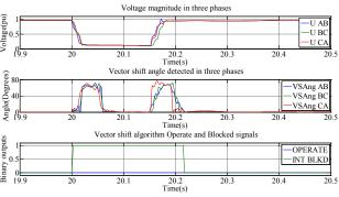
Figure 9. Vector shift algorithm behavior during A-B-C fault at the beginning of the adjacent MV feeder
