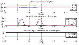
Figure 7. Vector shift algorithm behavior during A-G fault in the middle of the same MV feeder
