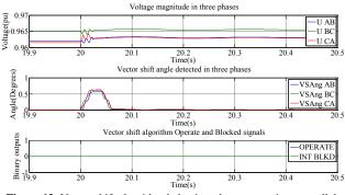
Figure 12. Vector shift algorithm behavior when connecting a parallel transformer
