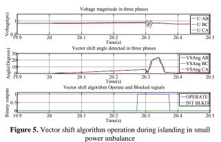
From Figure 5, it can be seen that after islanding at 20.0 s, the vector shift angles start to increase in all three phases. After the detected vector shift angle has increased above the pick-up setting, the algorithm issues an OPERATE pulse output at around 20.25 s, because no blocking conditions have been activated.
