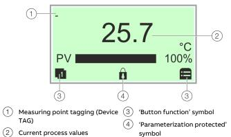
Figure 23: Process display (example)
