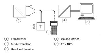
Figure 20: Example of FOUNDATION Fieldbus® interface connection
