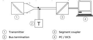
Figure 19: Example of PROFIBUS PA® interface connection
