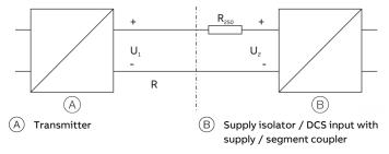
Figure 17: HART load resistance
