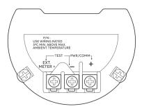
Figure 32: Terminals FSx430 (without binary output)
