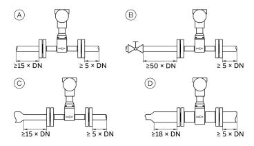
Figure 11: Straight pipe sections
