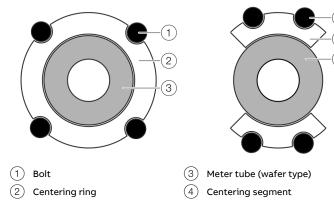
Figure 26: Centering the wafer type design with the ring or segment
