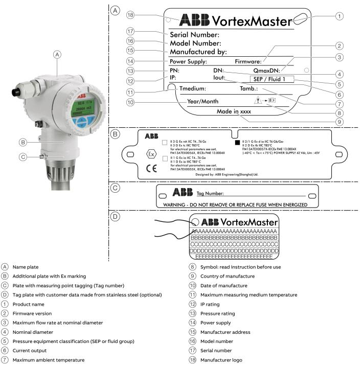
Figure 7: Types and tag plates (example)
