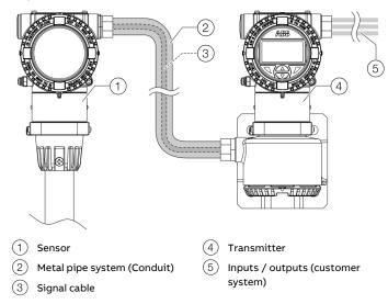
Figure 1: Signal cable installation with FM/CSA
