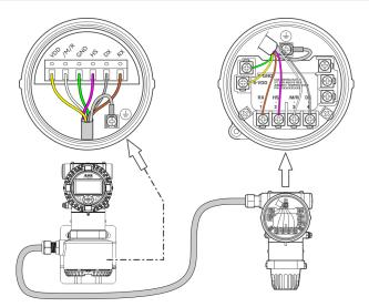
Figure 44: Electrical connection
