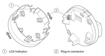
Figure 28: Rotating the LCD indicator
