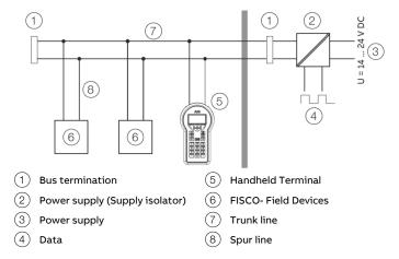
Figure 3: FISCO Control drawing (example)
