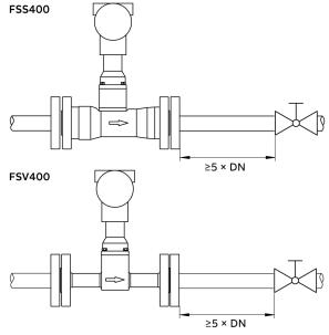
Figure 15: Installation of setting devices
