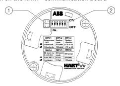
(1) Interface for LCD indicators and (2) DIP switch service port
