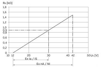
The voltage  $\rm U_S$  = 12 V is based on a load of 0  $\Omega.$
