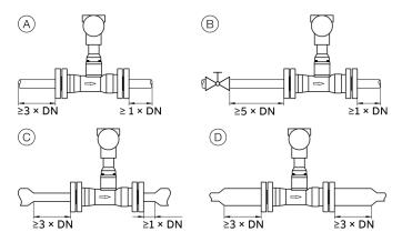
Figure 9: Straight pipe sections
