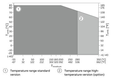
Figure 17: Measuring medium temperature  $T_{medium}$  dependent on the ambient temperature  $T_{amb.}$
