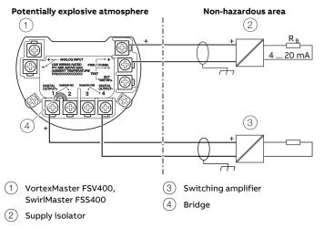
Figure 2: Electrical connection (example)
