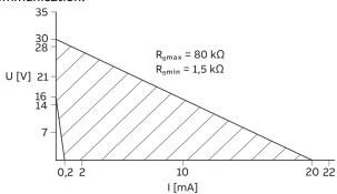
Figure 45: Range of the external supply voltage and current
