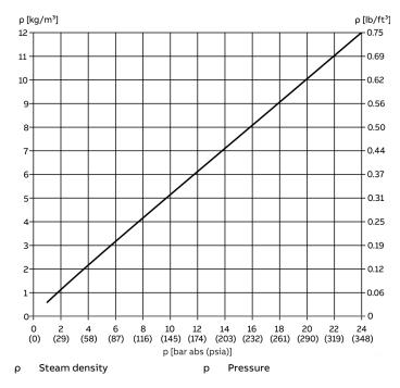
Figure 53: Saturated steam density by pressure
