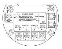
Figure 33: Terminals FSx450 or FSx430 with binary output
