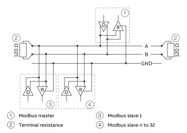
Figure 41: Modbus network (example)
