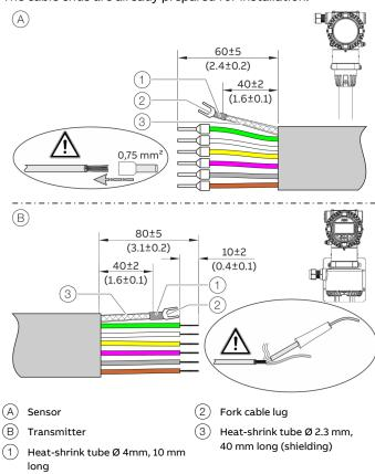
Figure 43: Signal cable, dimensions in mm (in)
