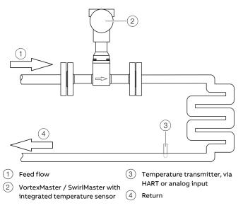
Figure 50: Measuring the energy of liquids
