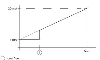
Figure 35: Behavior of the current output
