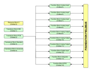
Figure 58: Design of the function blocks
