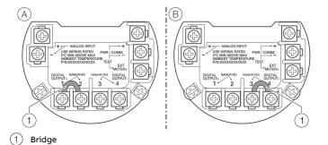
Figure 46: Hardware configuration of the digital output
