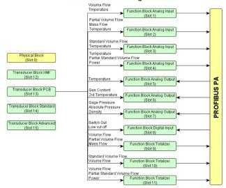
Figure 57: Design of the function blocks
