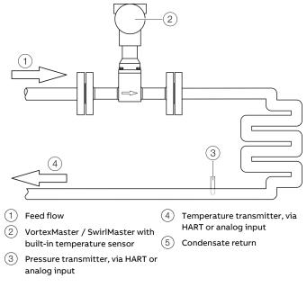
Figure 51: Energy measurement
