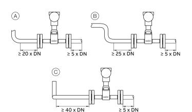
Figure 12: Pipe sections with pipe elbows
