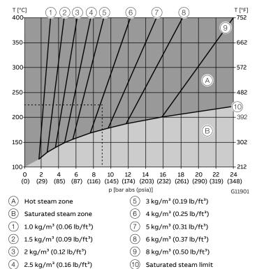
Figure 54: Steam density for hot steam The parallel lines (1) to (9) are lines of the same density.
