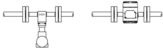
Figure 13: Installation at high measuring medium temperatures
