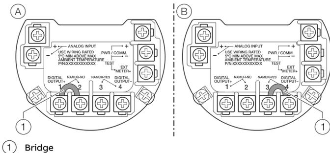
Figure 46: Hardware configuration of the digital output
