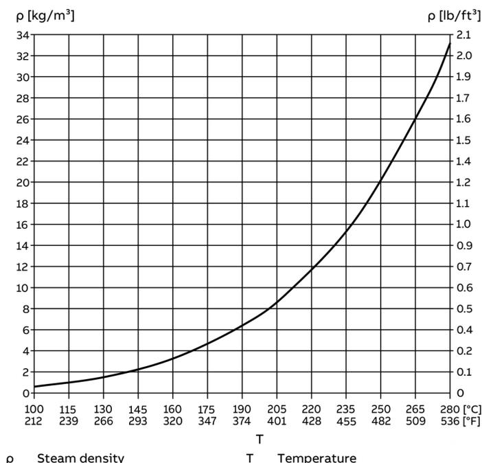
Figure 52: Saturated steam pressure by temperature
