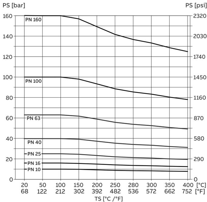
Figure 23: DIN flange process connection
