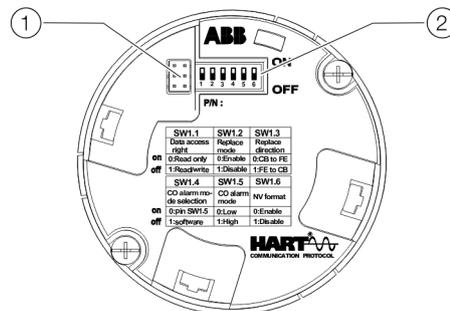
① Interface for LCD indicators and service port      ② DIP switch service port
