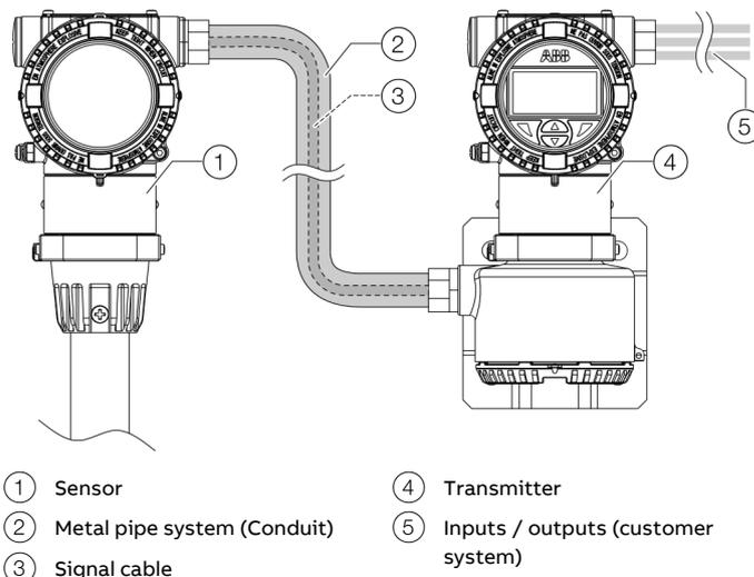
Figure 1: Signal cable installation with FM/CSA
