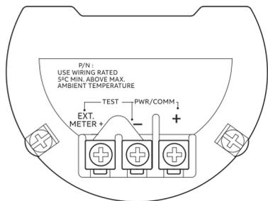
Figure 32: Terminals FSx430 (without binary output)
