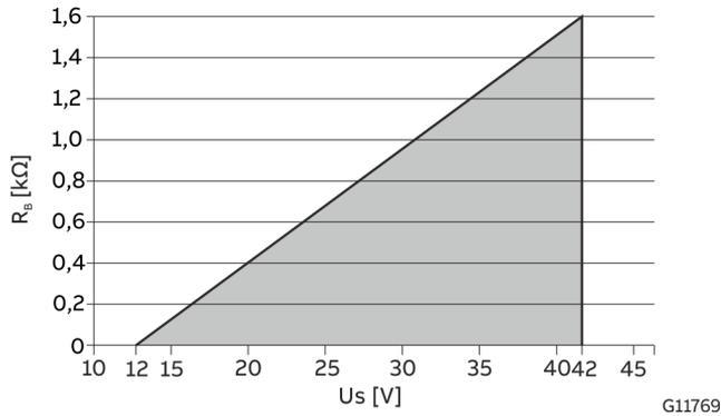
Figure 34: Load diagram of current output; load depending on supply voltage
