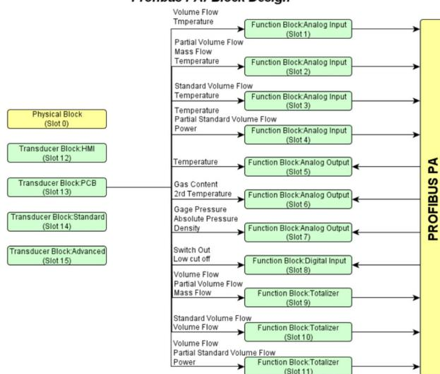
Figure 57: Design of the function blocks
