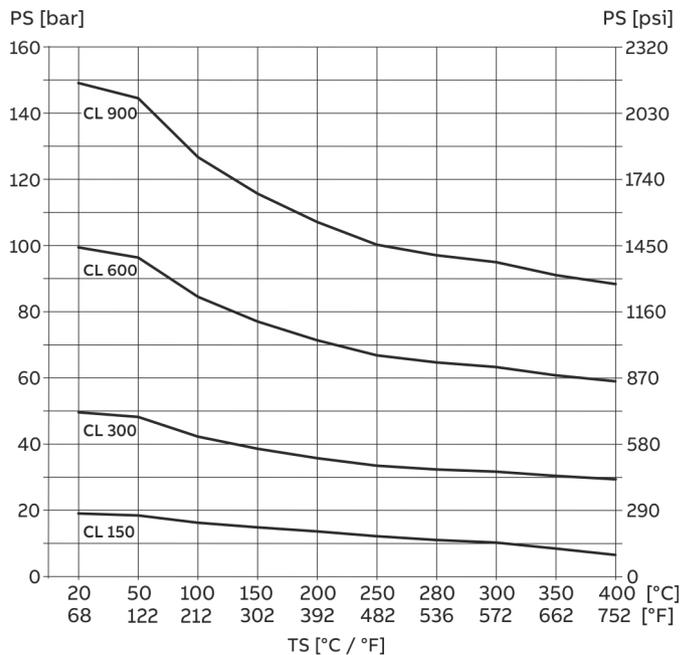
Figure 24: ASME flange process connection
