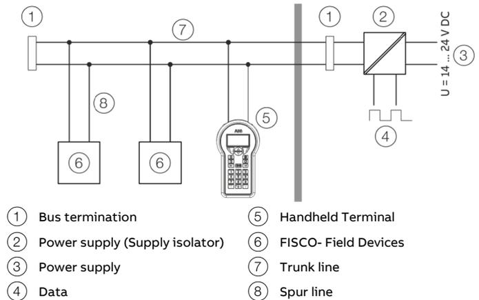
Figure 3: FISCO Control drawing (example)
