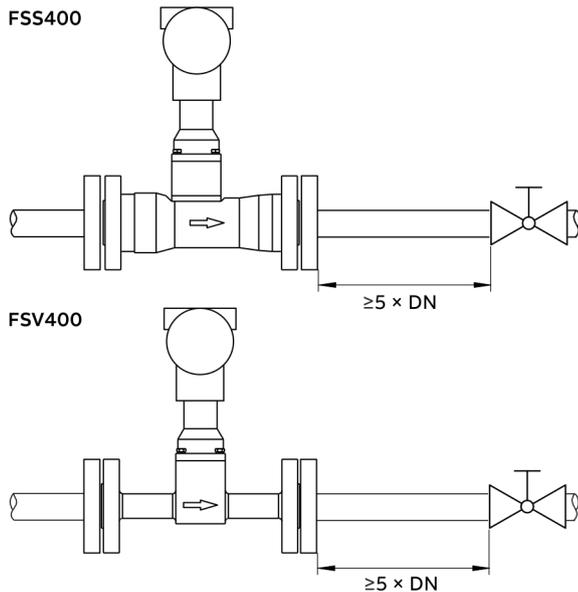
Figure 15: Installation of setting devices
