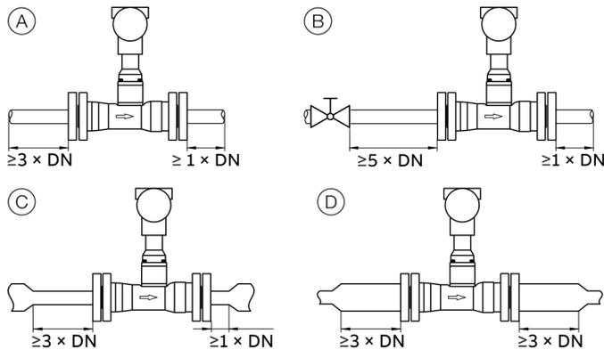
Figure 9: Straight pipe sections
