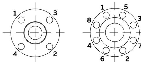
Figure 25: Tightening sequence for the flange screws
