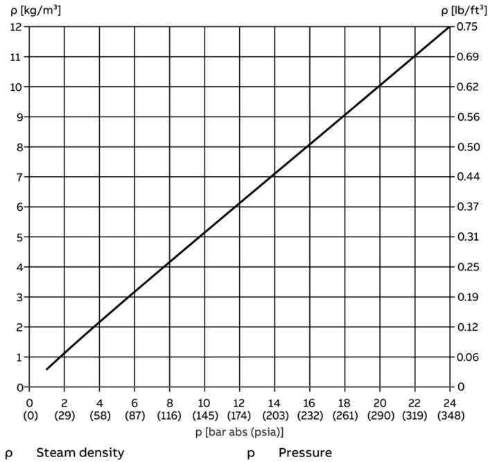
Figure 53: Saturated steam density by pressure
