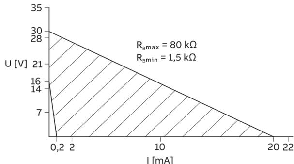
Figure 45: Range of the external supply voltage and current
