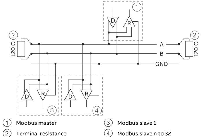
Figure 41: Modbus network (example)
