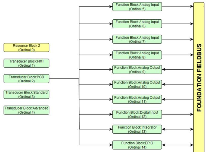
Figure 58: Design of the function blocks
