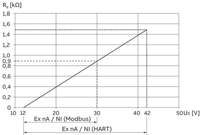
The voltage  $U_S = 12$  V is based on a load of  $0 \Omega$ .
