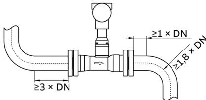
Figure 10: Pipe sections with pipe elbows
