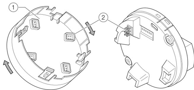
① LCD indicator                      ② Plug-in connector
