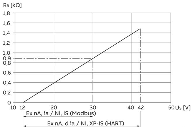
The voltage  $U_S = 12 \text{ V}$  is based on a load of  $0 \Omega$ .
