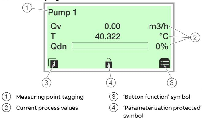
Figure 60: Process display (example)
