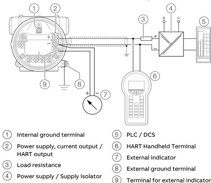
Figure 38: HART communication (example)
