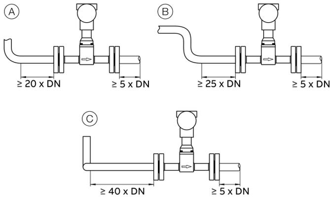
Figure 12: Pipe sections with pipe elbows
