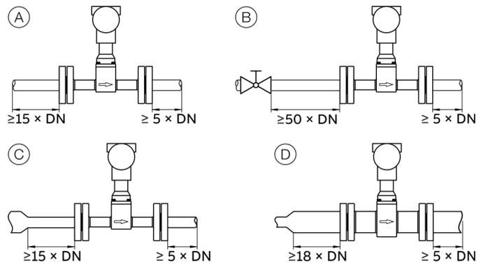
Figure 11: Straight pipe sections
