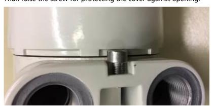
The W&M Sealing can be realized by installing a seal over the small gap between the cover and the lower housing. See the example below.
