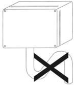
When laying the sample gas line, avoid the formation of water locks, particularly at the sampling points.
