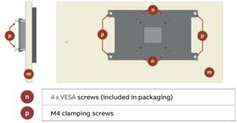
Tighten the M4 clamping screws P on the bracket to apply appropriate pressure to secure the device against the panel door and Wire up Power and Ethernet connections.
