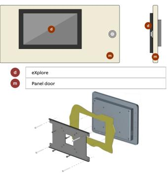
Place the back plate against the back of the **eXplore** unit and reinsert the 4 x VESA screws.
