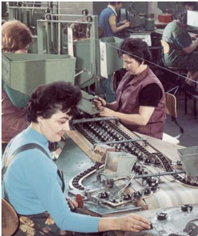
1965 Assembly-line production Busch-Duro 2000® switch base
