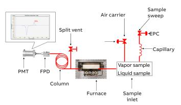
Figure. 2 Operating diagram of the analysis system (sample injection, oxidation, separation, measurement)
