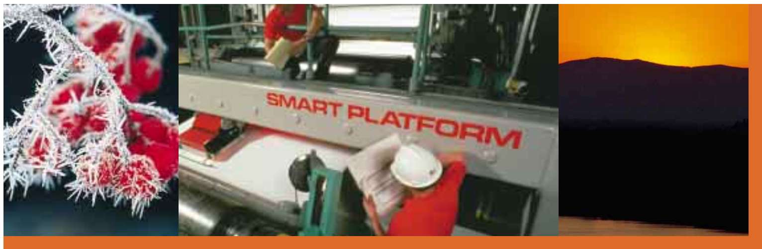
The ABB Smart platform sensors measure and control a moving paper web 1,200 times per second. Fletcher paper, Alpena, Michigan, USA.
