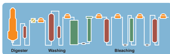
ABB Autobleach control system monitors the color of the fibers throughout the bleaching process.
