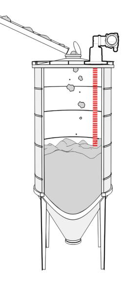
The LLT100 provides a unique and reliable level measurement solution for a variety of sugar level applications such as inventory measurement for sunflower-bagasse in conical and tall silos. There's no mapping or any adjustments of the various angles of repose or material dielectrics.
