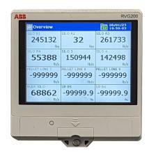
The ABB RVG200 can plot the level signal as (Pv), but also output alarms based on low or high values. It can also calculate the volume based on basic dimensions and formulas that are preprogrammed into the recorder.
