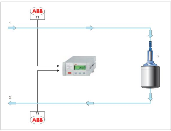
Fig. 4-1: Function diagram of differential temperature measurement
