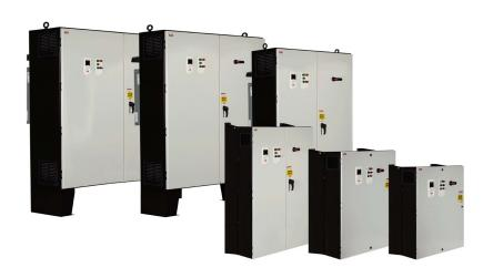
The ACS880-PE Enclosed Drive features a single ACS880-01 flange-mounted variable frequency drive in a wall-mounted or floor-standing enclosure and is available in a UL type 1 or type 12 design. It also features a wide selection of optional components including a manual two-contactor bypass with or without a soft start and a variety of power filters.
