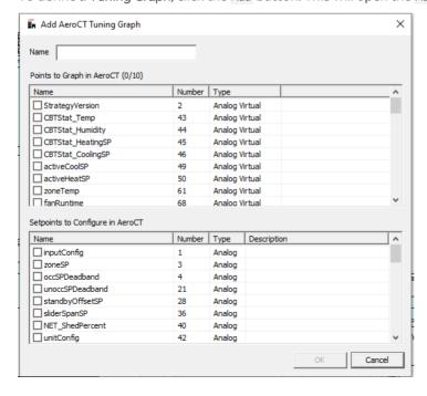
The Add AeroCT Tuning Graph dialog lists all BACnet exposed Virtual and Hardware points in the strategy. Up to 10 Points can be selected to Graph in the Aero<sup>CT</sup> application
