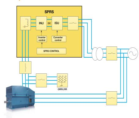
A slip ring motor starts by the direct-on-line method with grid rotor resistance (GRR) connected to rotor. After the motor achieves the desired speed, control can be shifted to SPRS by auto or manual operation.
