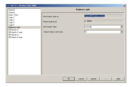
The parameter *Send output value* as is now firmly adjusted to 2-byte [EIB floating comma].
