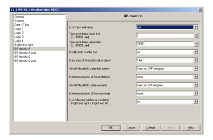
The Tolerance band is now adjustable for the lower and upper limit of 0...99.000 Lux.
