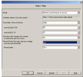
The parameter Date/time delayed send after bus voltage recovery, mains voltage recovery and was changed in
