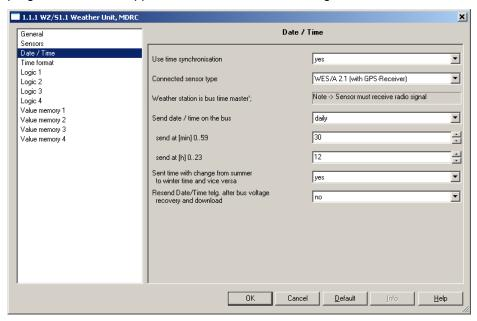
In the parameter window *Date/Time* was inserted additionally the parameter *Connected sensor type*.
