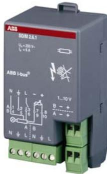
The Switch/Dim Actuator Module is operated in a module slot of the Room Controller Basis Device. It dims electronic ballasts with a 1...10 V interface. The device has two independent outputs for dimming two groups of luminaires. One relay contact per channel is used to switch the lighting circuit on/off.
