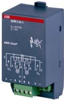
The 2-fold Shutter Actuator Module is a device for insertion in the Room Controller Basis Device. Using relay contacts, it switches two independent electric drives such as shutter motors or ventilation flap drives. The nominal switching voltage is 12 or 24 V DC.
