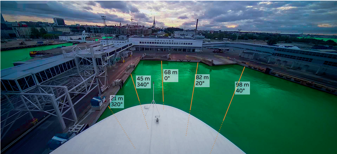
Figure 5: A sequence taken from the lookout camera of MS Finlandia while leaving one of Tallinn's ports. The water clearance map and the directional clearances are computed in real time from the camera stream.
