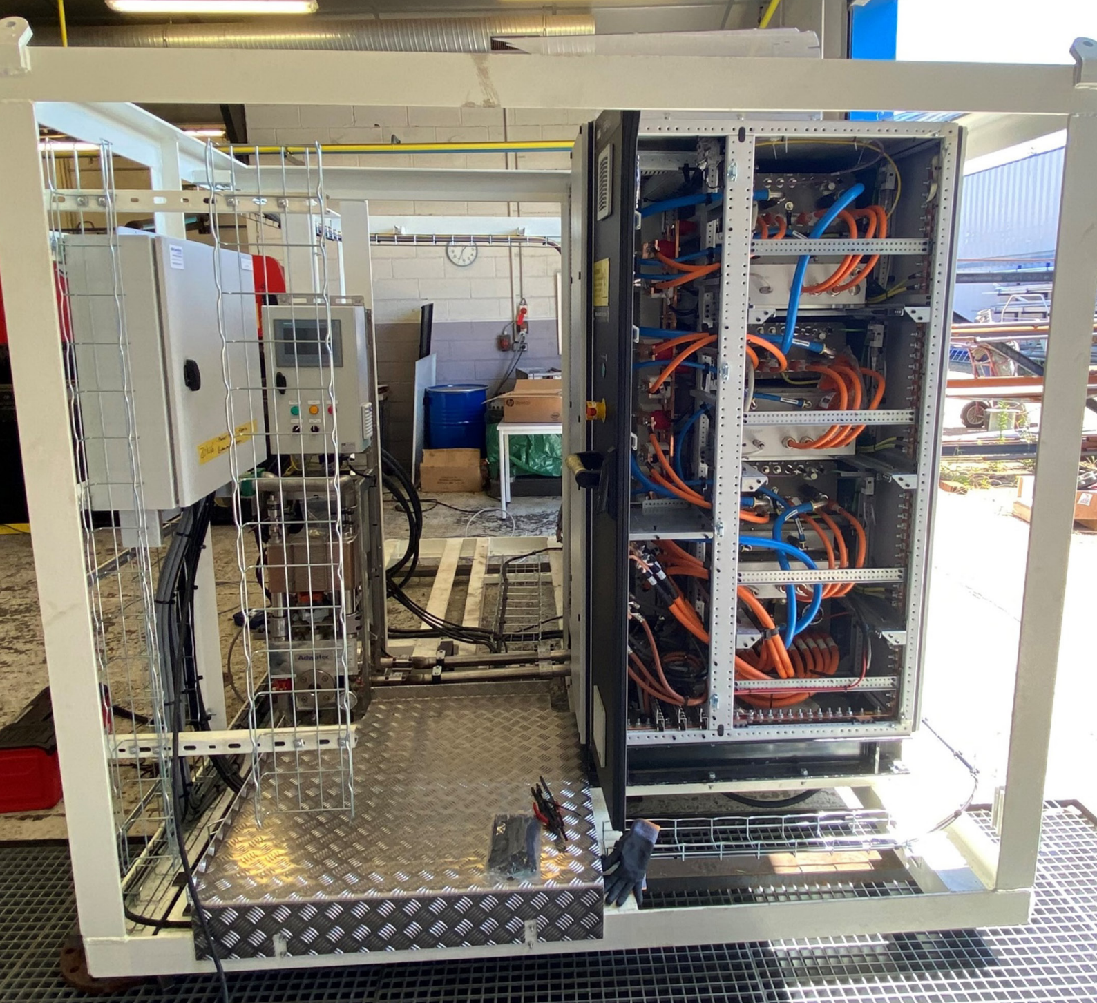
Figure 5: Fuel cell and battery power train skid installation
