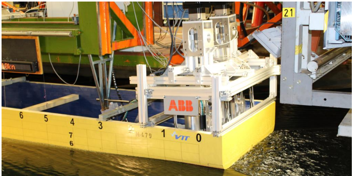
Figure 4: Self-propulsion test with two ABB Dynafin™ units retrofitted to a PSV hull model
