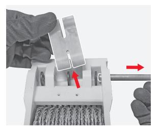
Manually remove the insulation protection.
