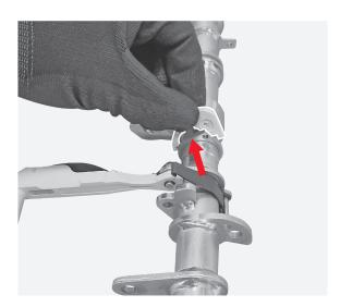
By means of 2 flat screwdrivers remove the benzing.
