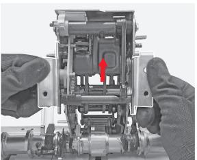
**188**Manually remove the operating mechanism.
