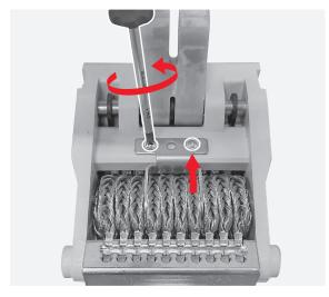
By means of the flat screwdriver push the pin as indicated by the arrow.
