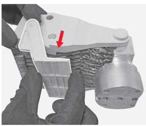
Place the mobile contact assembly as shown in the picture and then by means of the hammer and of the rod push out the pin.
