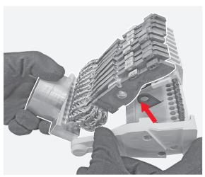
Manually remove the contacts spacer.
