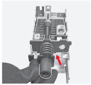
By means of the flat screwdriver remove the benzing and after manually remove the feeler.
