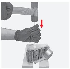
Manually separate the mobile contact from its contacts holder.
