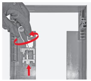
By means of the flat screwdriver remove the 2 benzings mounted on the T.U. Reset assembly.
