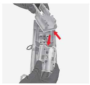
214 Manually remove the protections from the pole.
