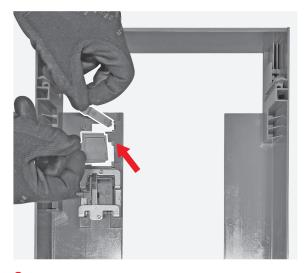
9 Manually remove the T.U Reset assembly.
