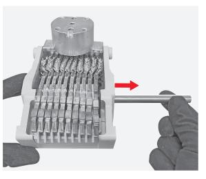
**249**Manually unhook both appendixes of the insulation protection.
