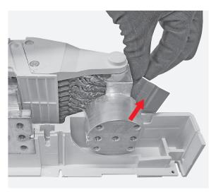
Manually remove the mobile contact.
