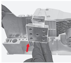
**245**By means of the cross screwdriver unscrew the 2 screws fixing the jumper to the mobile contact assembly.
