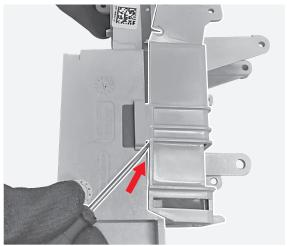
By means of the flat screwdriver unhook as indicated by the arrow the flat cover from the MID main structure.
