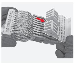
Manually remove the 10 springs mounted on the contacts holder.
