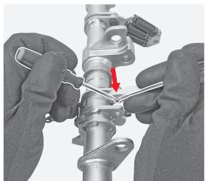
Manually remove the lever.
