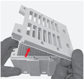
**229**By gravity let the 2 filters and the spacer separate from the arching chamber shell.
