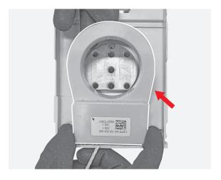
Manually unhook the cable from the sensor.
