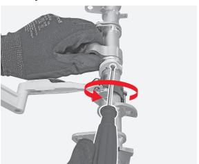
Manually remove the cam.
