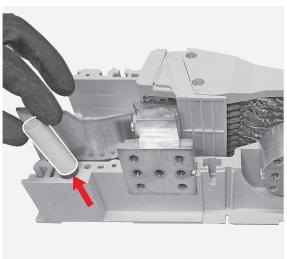
Manually remove the insulating protection.
