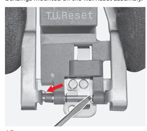
**12**By means of the torx key remove the 2 screws fixing the plug to the circuit breaker front cover.
