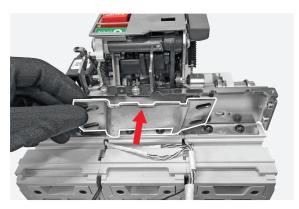
Manually remove the upper cross beam.
