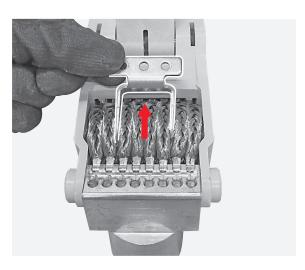
Manually remove the pin and the tie rod.
