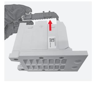
Manually separate the arc quenching and the plate.
