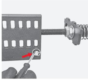
**115**By means of the flat screwdriver remove the benzing.
