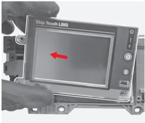
By means of the cutter start removing the trip unit front label and by means of the pliers complete the operation.
