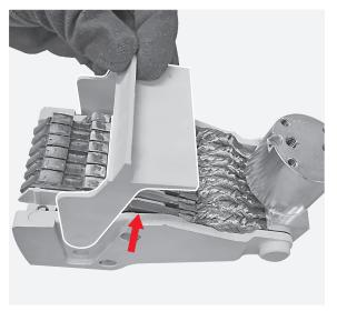
By means of the flat screwdriver push the pin as indicated by the arrow.
