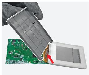
Manually separate the gasket from the display.
