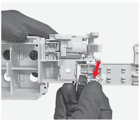
By means of the flat screwdriver slightly lift up the appendix as indicated by the arrow and manually remove the trip coil assembly.
