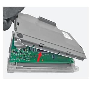
**58**By means of the flat screwdriver remove the battery cover on the left side of the display.
