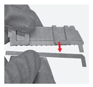
**218**By gravity let the plates come out from the arching chamber main structure.
