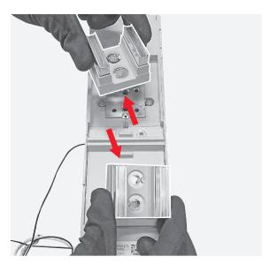
**200**Manually separate the terminals and their protections.
