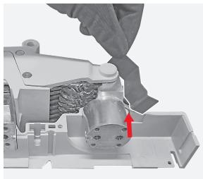
Manually remove the arc deflector protection present on the fixed contact.
