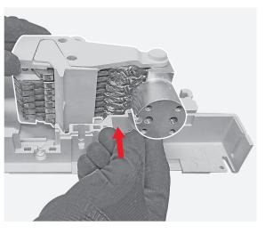
Manually remove the insulating protection.
