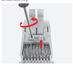
Manually remove the jumper.
