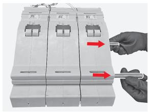
By means of the flat screwdriver unscrew the screws fixing the 3 wires connecting the measuring module connector to the sensors mounted inside the poles.
