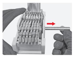
Manually remove the contacts spacer.
