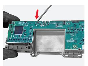
**76**Manually remove trip unit printed circuit board.
