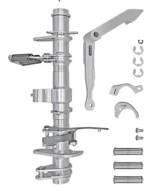
**187**By means of 2 flat screwdrivers remove the benzing.
