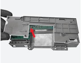
**75**By means of the flat screwdriver unhook the trip unit printed circuit board.
