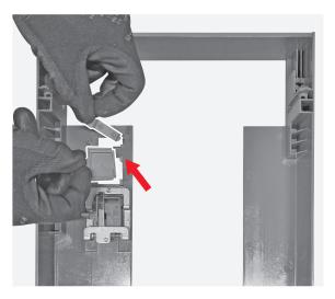
**9** Manually remove the T.U Reset assembly.
