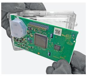
By means of the flat screwdriver remove the "i TEST" pushbutton from the HMI LCD cover.
