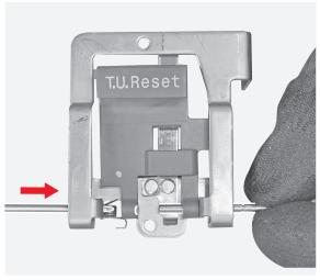
By means of thr torx key unscrew the 2 screws fixing the T.U. Reset assembly to the front cover.
