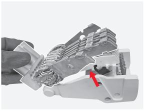
Manually remove the 8 springs mounted on the contacts holder.
