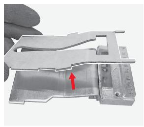
By means of the cross screwdriver unscrew the 2 screws fixing the jumper to the mobile contact assembly.
