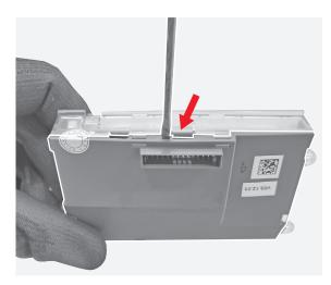
Manually separate the display and the HMI LCD cover,
