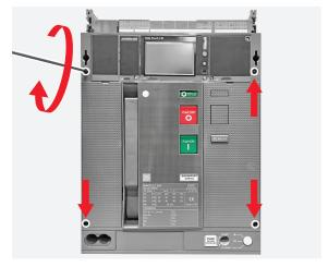
By means of the torx key unscrew the 2 screws fixing the 2 plugs to the front cover.
