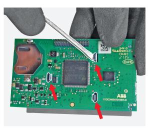
Manually separate the display from its printed circuit board.
