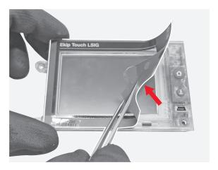
Manually remove the battery.
