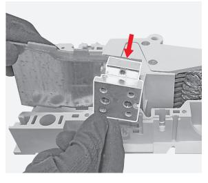
Manually remove the mobile contact.
