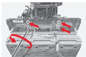
By means of the torx key unscrew the 6 screws fixing the upper cross beam to the circuit breaker main structure.
