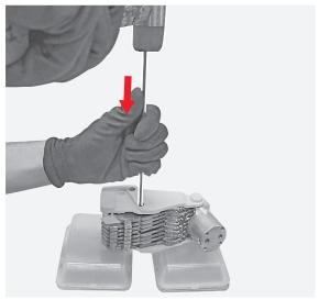
Manually remove the pin.
