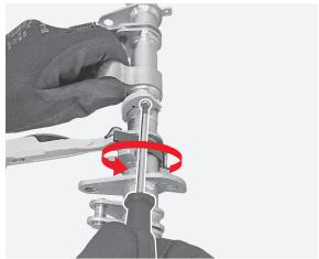
**186** Manually remove the cam.
