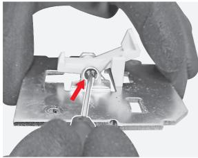
By means of the flat screwdriver push the pin as indicated by the arrow and let the spring and the CD block cover separate from the cover.
