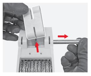
Manually remove the insulation protection.
