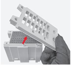
**221**By gravity let the 2 filters and the spacer separate from the arching chamber shell.
