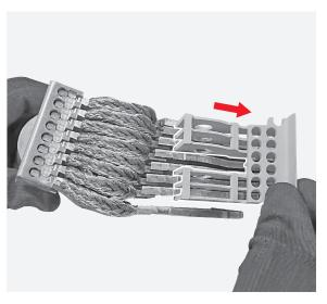
**250**By means of the flat screwdriver slightly push the shoulders located at the sides of the contacts holder and after manually push the shoulder located in the middle.
