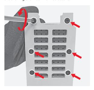
Manually remove the arching chamber cover
