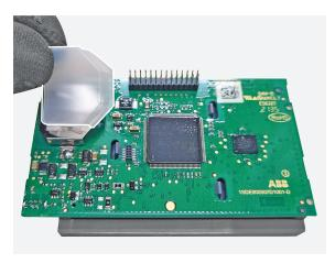
Manually remove the display support.
