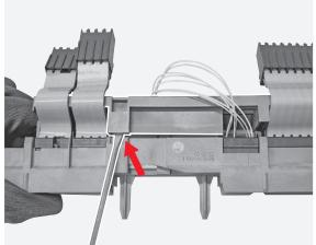
By means of the flat screwdriver unhook the right side wall from the sliding contacts main assembly as indicated in the picture.
