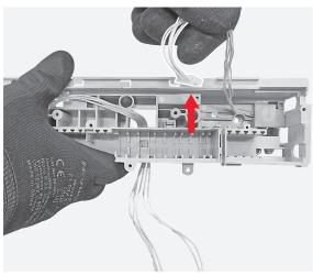
By means of the flat screwdriver unhook the 2 microswitches from their support and after separate the microswitches support from the rest of the connector.
