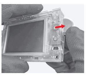
Manually remove the HMI box from the display.
