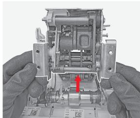
**179** Manually remove the operating mechanism.
