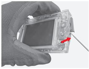
**60**By means of the flat screwdriver unhook the HMI box from the display.
