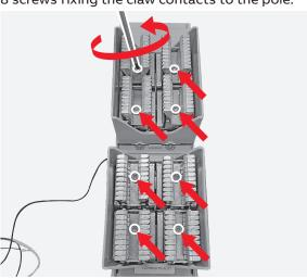
Push the claw contacts as indicated by the arrows and after manually remove the claw contacts.
