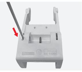
Manually separate the mobile contact from its contacts holder.
