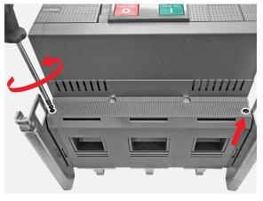
Manually complete the removal of the withdrawable terminals cover.
