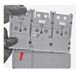
**160** Manually remove the 3 arching chambers.
