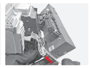
By means of the flat screw driver unhook the white connector from the trip unit.
