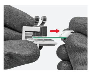
Manually remove the printed circuit board.
