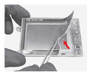
**76** Manually remove the battery.
