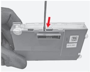
Manually complete the removal of the HMI box.
