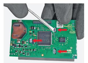
Manually remove the display support.
