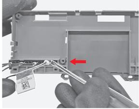
By means of the cutter start removing the 2 labels located on the trip unit back cover and by means of the pliers complete the operation.
