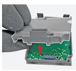
Manually remove the printed circuit board from the Ekip measuring blind cover.
