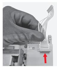
By means of the flat screwdriver push the appendix as indicated by the arrow and after manually remove the 2 couples of auxiliary contacts lifting them up.
