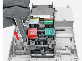
Close the circuit breaker pushing the close button.
