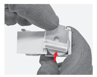
By means of the flat screwdriver push out from the trip coil group the trip coil.
