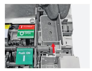
118 Manually remove the connector located in the upper part of the MID.
