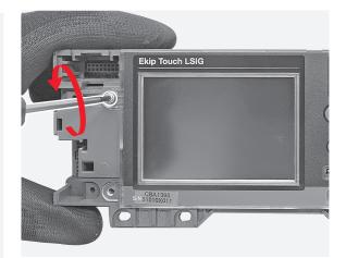
By means of the flat screwdriver unhook the display from the trip unit main structure.
