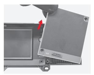
By means of the cutter start removing the label located on the Ekip measuring blind plug and by means of the pliers complete the operation.
