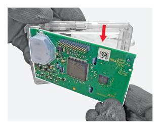
**82** Manually remove the battery gasket.
