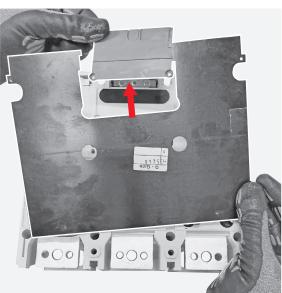
By means of the flat screwdriver clean from silicone rear part of the breaking part main structure.
