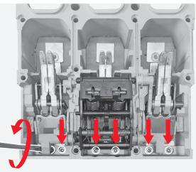
Manually pull the shaft as indicated by the arrow and by means of the flat screwdriver remove the 3 benzings.
