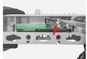
Manually remove the trip coil.
