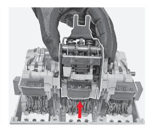
Manually remove the S51 and SR levers mounted on the mobile contacts assembly.
