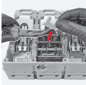
**33**Manually remove the arching chambers.
