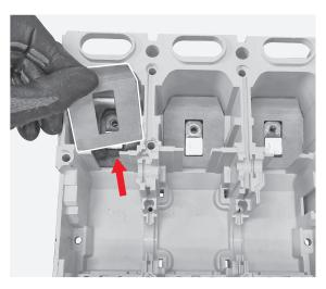
Manually pull the main fixed contacts as indicated by the arrow, slightly lift them and after manually complete the removal.
