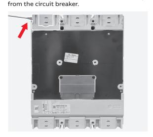
4 Insert the flat screwdriver as shown in the picture and unhook the cap kits from the circuit breaker.
