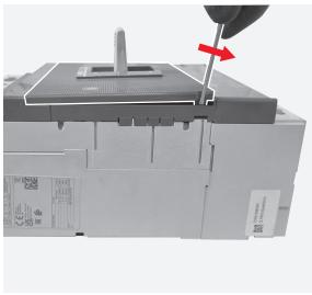
**7**Manually remove the aesthetic front cover.
