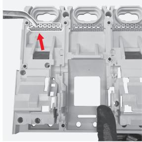
By means of the flat screwdriver remove the 2 shock absorbers located at both sides of the breaking part cover.
