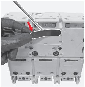
By means of the flat screwdriver clean from silicone rear part of the breaking part main structure.
