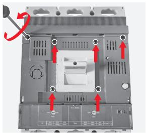
Manually remove the upper and the lower front covers.
