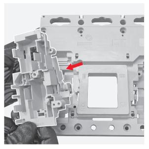
By means of the pliers remove the 3 grids located in the upper part of the breaking part cover
