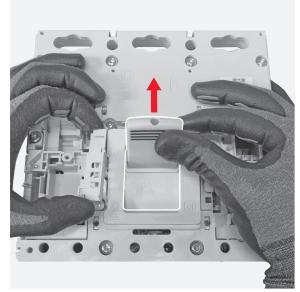
**17**By means of the pliers remove the spring mounted inside the AUE lever group.
