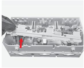
Manually remove the 2 pins mounted inside the trip shaft.
