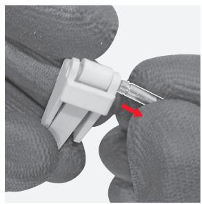
Manually remove the lever DX assembly located on the right part of the breaking part.
