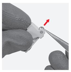
**25**Manually separate the pin, RC lever release and the RC lever support.
