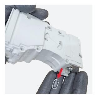
39 By means of the pliers remove the silicone sheath located in the bottom part of the pole.
