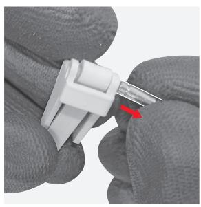
Manually remove the lever DX assembly located on the right part of the breaking part.
