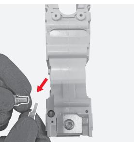
**38**By gravity let the pin fall down from the pole.
