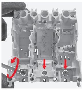
**34**Manually separate the plastic part from the metals parts constituting the terminals connections removed at previous step.
