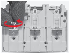
**55**By means of the flat screwdriver lift the top cover of the trip unit and manually complete the removal.
