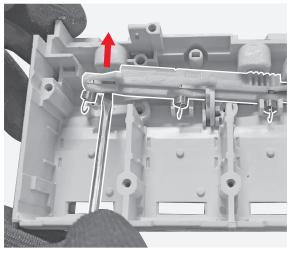
**72** By means of the pliers remove the 3 springs.
