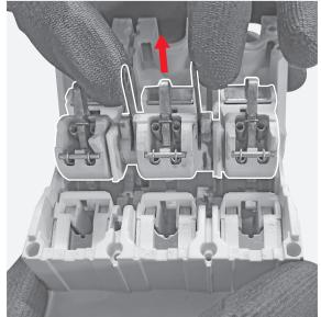
**39**By means of the pliers remove the 2 plugs mounted on the moving contacts assembly\*.
