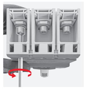
2 Insert the flat screwdriver as shown in the picture 2 and push it up in order to remove the cap kits.
